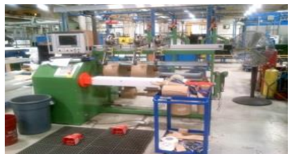
Automated Coil Winding
